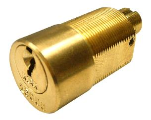
The Camlock is a compact, threaded cylinder interlock designed to fit smaller-sized switchgear. The key is trapped or released according to the position of the cam. It is designed to be installed with provisions or bracketry provided by the breaker manufacturer. The Camlock can be linked to other camlocks with the proper bracketry.
